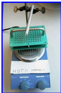
Photo 1: sterilization of the replicator on a hot plate: the alu bar presses the grip down and so ensures that all pins are well in contact with the hot plate.
