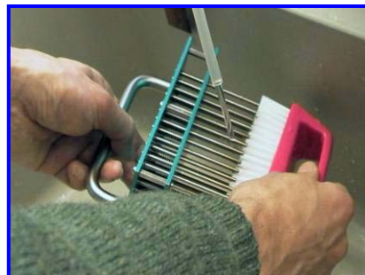
Photo 2: washing of the replicator using demineralized water: it is important that all cell debris is well removed before sterilizing and using the replicator again. It is advisable to avoid wetting the aluminum plates or the springs during washing.
