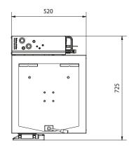
Inner chamber stainless steel, outer chamber PUR (insulation), door polycarbonate
