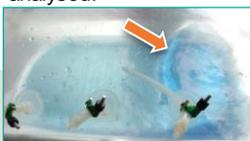
Example of the wave while shaking (4 L, 25 rpm). This kind of wave results in a good mixing time.
